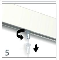
Twist&turn both Twister wires out of the rail.
