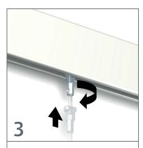
Twist&turn both Twister wires in of the rail.
