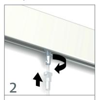
Twist&turn both Twister wires with hook in the rail.
